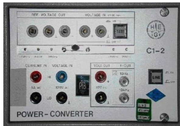
Figure 1. Front panel of the travelling standard MTE C1-2.
